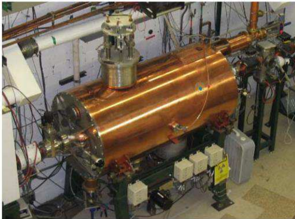
Figure 4.2: A schematic and photograph of the RFFS. The beam enters the chamber at left, experiences deflection according to the electric field throughout its flight between the two electrode plates, and exits to the right. The RF coupler at top is used to couple the oscillation frequency of the RFFS to that of the cyclotron. This figure is reproduced from the original RFFS paper, Ref. [66].
